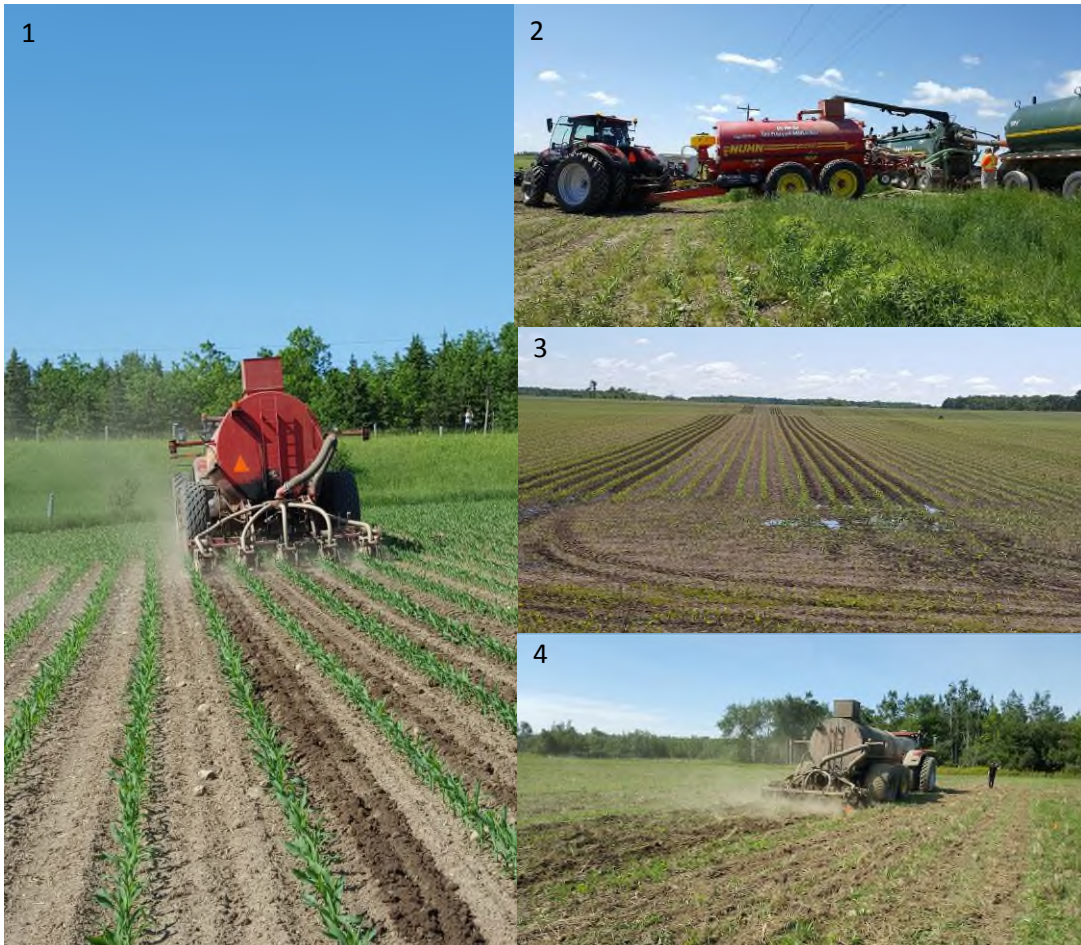
Figures 1-4: 1. Side-dress application of amendment Site 2, 2. Transfer of digestate to tanker applicator, 3. post application plot strips Site 1, 4. application into cover crops and winter wheat stubble.
